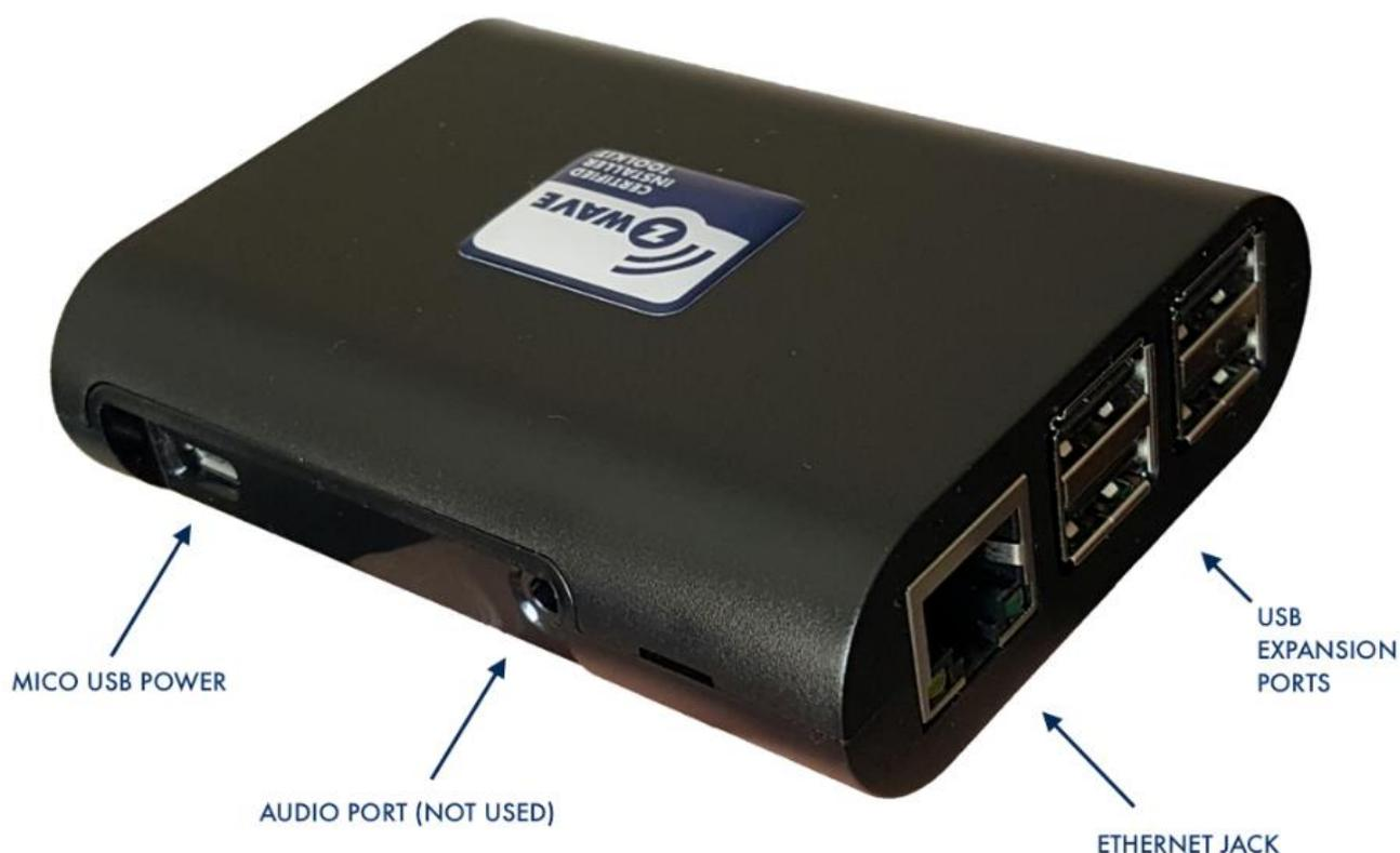
The tool requires power through the Micro USB Power jack located on the side of the unit. Plug a micro USB power adapter into the jack to use the unit. If you need to use the CIT while mobile, you may use a mobile power pack such as the ones used to power mobile phones.
