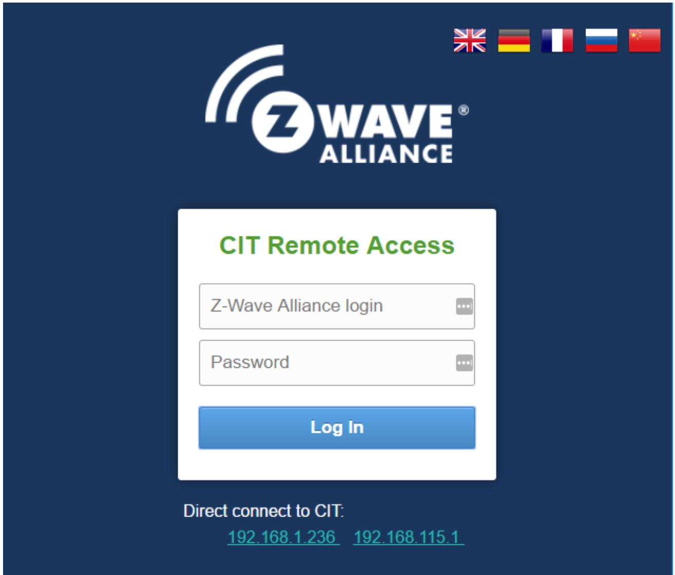
If your CIT was found, it will display two IP addresses as hyperlinks. The first IP address is the CIT's address on your local (customer) network – the Ethernet jack network. The second IP address is the CIT's built-in WiFi address. Click on the first hyperlink – in the example above, it would navigate to <http://192.168.1.236:8083> (The IP address vended on your customer network will vary)
