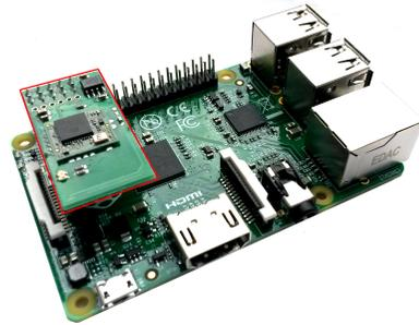
Thank for you buying **RaZberry** that turns your Raspberry Pi into a Z-Wave enabled Home Gateway. The solution consists of two parts: (A) the transceiver hardware that is plugged on top of the RaZberry on as shown in the image above (it uses the GPIO Pins 1-10), (B) a Z-Wave controller software running on the Raspberry Pi itself. You can download a free license of Z-Way from the website [razberry.z-wave.me](http://razberry.z-wave.me) that will work with the hardware out of the box.
